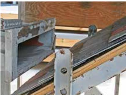
*Wind is directed by the test apparatus horizontally into the panel with the target area being the third course up from the bottom of the panel at a distance of 7 inches.*
