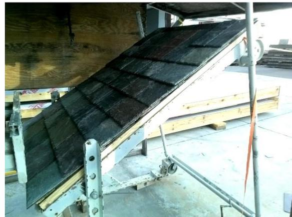
Deck #2: At End of Testing (160 mph)
