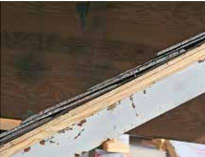
*After successful completion of testing on both panels at 150 mph we increased the wind speed to the maximum 160 mph that the test apparatus was capable of producing for 10 minutes. Once again, with the exception of the upper unrestrained course, both panels remained intact and very stable throughout the wind speed increases and intervals to 160 mph. On examination after the test, both panels exhibited no damage, displacement or blow off of any kind.*
