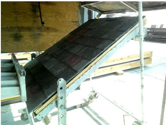
Deck #1: At End of Testing (160 mph)
